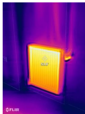
Figure 3- Thermal imaging shows radiators heat up
